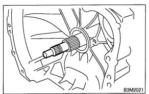
3) Extract the oil pump shaft from torque converter clutch.
