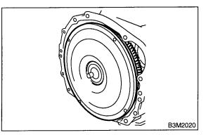
2) Remove the input shaft.
