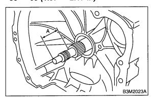
4) Holding the torque converter clutch assembly by hand, carefully install it to the torque converter clutch case. Be careful not to damage the bushing. Also avoid undue contact between the oil pump shaft bushing and stator shaft portion of the oil pump cover.
