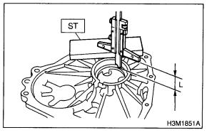
2) Measure the distance " $\ell$ " from the transmission case mating surface to end of bearing with ST.
