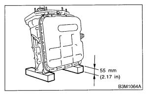
12) Remove the oil pan and control valve body.<Ref. to AT-83 REMOVAL, Control Valve Body.>13) Remove the oil pump housing.
