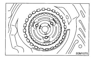
20) Take out the thrust needle bearing, planetary gear assembly and the low clutch assembly.
