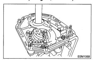
15) Install the control valve body and oil pan. <Ref. to AT-84 INSTALLATION, Control Valve Body.>
