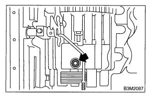
8) After all 2-4 brake component parts have been installed, blow in air intermittently and confirm the operation of the brake.
