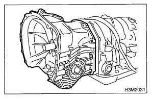
11) Place two wooden blocks on the workbench, and stand the transmission case with its rear end facing down.
