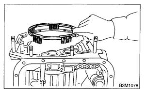
4) Position snap ring in transmission. Using ST, press the snap ring into place. ST 498677100 COMPRESSOR
