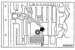
15) Take out the high clutch and reverse clutch assembly. <Ref. to AT-89 REMOVAL, High Clutch and Reverse Clutch.>
