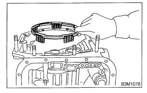
23) Take out 2-4 brake piston and piston retainer.
