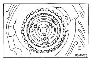
7) Install 2-4 brake oil seal to transmission case. NOTE:
