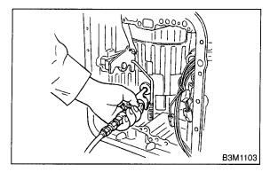
9) Measure the clearance between the retaining plate and the snap ring.
