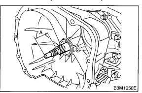
23) Install the torque converter clutch assembly. <Ref. to AT-34 INSTALLATION, Torque Converter Clutch Assembly.>
