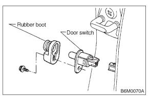
2) Move switch and check continuity between terminals of door switch.
