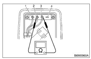
$\widehat{\text{_{CHECK})}}$ : Is the resistance less than 1  $\Omega$ ?
