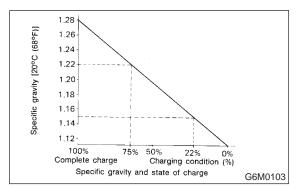
(2) Measuring the specific gravity of the electrolyte in the battery will disclose the state of charge of the battery. The relation between the specific gravity and the state of charge is as shown in the figure.
