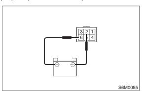
2) Check wiper motor operation at high speed: Connect battery wiper motor. Check wiper motor for proper operation at high speed.
