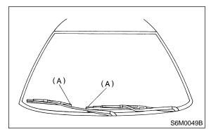
3) Adjust washer ejecting area on windshield glass as shown in the figure when vehicle stops.
