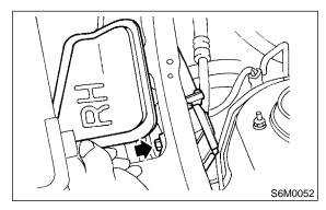
6) Remove bolts which secure sleeve unit.
