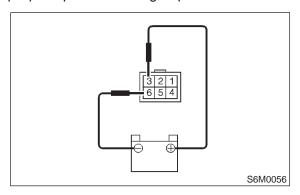
3) Check wiper motor for proper stoppage: Connect battery to wiper motor. After operating wiper motor at low speed, disconnect battery to stop it.
