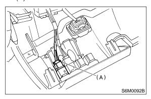
5) Remove main switch by pushing it outward.
