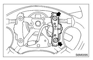
8) Disconnect horn and cruise control command switch connector, then remove cruise control command switch.
