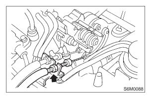
6) Disconnect cruise control vacuum hose from intake manifold.
