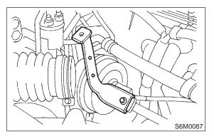
5) Remove cruise control cable end from throttle cam.
