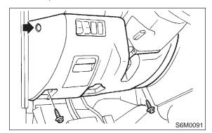
4) Disconnect connector from cruise control main switch (A).
