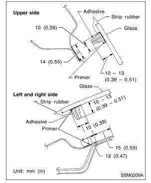
3) About one hour after installation, test for water leakage. Leave vehicle for 24 hours before using it.
