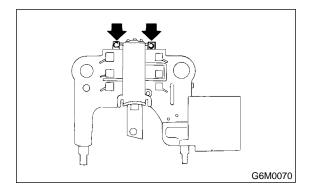
6) Remove the nut and insulating bushing at terminal B, and remove rectifier.
