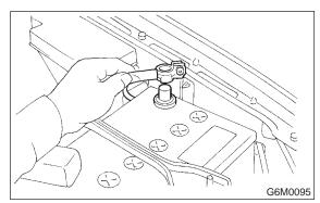
2) Disconnect connector and terminal from generator.
