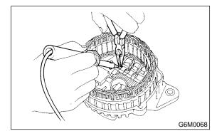
4) Remove screws which secure IC regulator to rear cover, and unsolder connection between IC regulator and rectifier to remove IC regulator.
