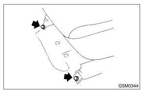
7) While disconnecting side airbag connector, detach front seat. (Side airbag equipped vehicle) <Ref. to 5-5 [M2F2].> and inner belt connector.
