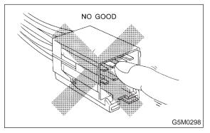
• When connecting or disconnecting airbag connector, make sure ignition switch is OFF.
