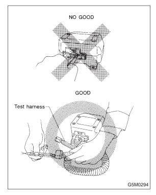
• Do not drop the airbag modulator parts, subject it to high temperatures over 90°C (194°F), or apply oil, grease, or water to it; otherwise, the internal parts may be damaged and its reliability greatly lowered.
