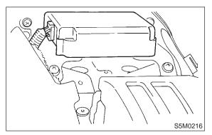
7) Disconnect body harness connector (B31) from airbag connector (AB1) located at front pillar lower (driver side). <Ref. to 5-5 [M2F3].>
