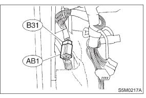
8) Disconnect front sub sensor connector (yellow) from airbag main harness located at front pillar lower (both sides). <Ref. to 5-5 [M2F5].>
