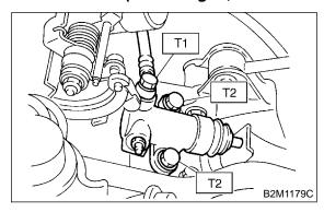
5) After bleeding air from operating cylinder, ensure that clutch operates properly. <Ref. to 2-10 [W2A0].>
