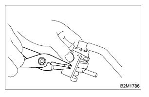
9) Disconnect vacuum hose from pressure control solenoid valve.
