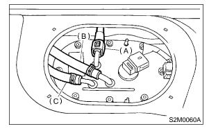
9) Remove nuts which install fuel pump assembly onto fuel tank.
