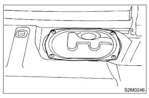
6) Disconnect connector from fuel pump.
