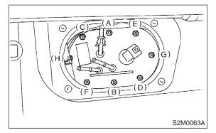
5) Connect connector to fuel pump relay.
