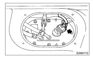
7) Move clips, and then disconnect fuel delivery hose (A), return hose (B) and jet pump hose (C).
