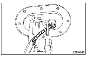
12) Remove bolt which installs fuel level sensor on mounting bracket.
