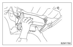
4) Disconnect connector from drain valve.
