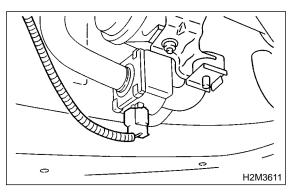
7) Disconnect evaporation hoses, and remove drain filter.
