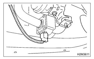
5) Disconnect evaporation hoses (A) from joint pipes.
