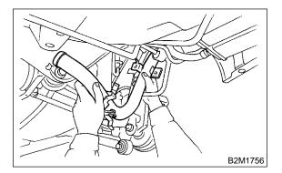
4) Disconnect evaporation hoses from shut valve.
