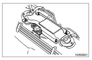
3) Move clips, and disconnect hoses from vent valve.
