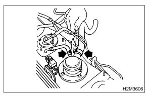
4) Remove nuts which install vent valve on fuel tank.
