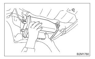
4) Disconnect connector from drain valve.
