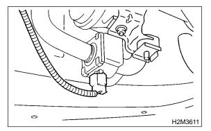
5) Disconnect evaporation hoses from drain valve.
