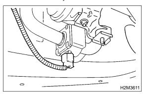
7) Move drain filter to upper side, and remove drain valve with bracket.
