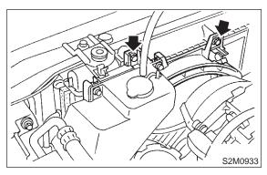
Tightening torque: 4.9±1.5 N⋅m (0.50±0.15 kg-m, 3.6±1.1 ft-lb)
