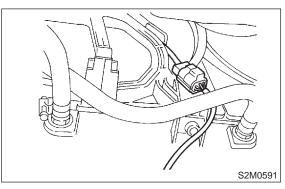
6) Detach ATF cooler hose attached to a clip under the radiator main fan shroud. (AT vehicles only)
