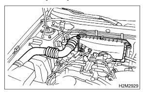
4) Disconnect front oxygen (A/F) sensor connector.
