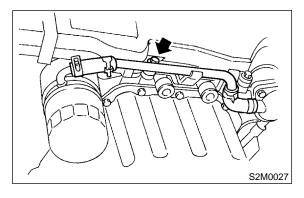
7) Remove water pipe and hoses between oil cooler and water pump. (AT vehicles only)
