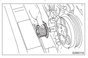
18) Remove bolts which install oil pump onto cylinder block.
