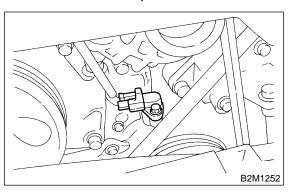
11) Remove camshaft position sensor. <Ref. to 2-7 [W10A0].>
