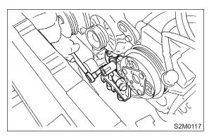
19) Remove oil pump using flat bladed screw-driver.
