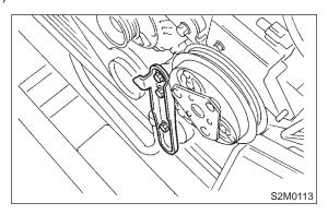
14) Remove crankshaft pulley using ST.ST 499977100 CRANKSHAFT PULLEY WRENCH
