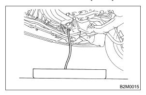
6) Remove bolts which install water pipe of oil cooler to oil pump. (AT vehicles only)
