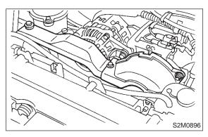
7) Connect connector and terminal to generator.
