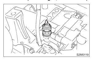
3) Connect terminal of oil pressure switch.
