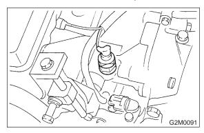
3) Remove oil pressure switch.
