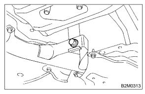
10) Remove front and center exhaust pipe assembly from the vehicle.
