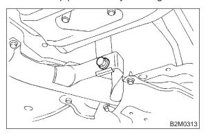
4) Tighten bolts which hold front exhaust pipe onto cylinder heads.
