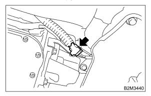
7) Separate front and center exhaust pipe assembly from rear exhaust pipe.
