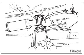
6) Tighten bolt which holds front and center exhaust pipe assembly to hanger bracket.
