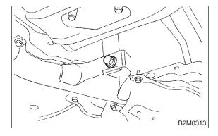
7) Connect rear oxygen sensor connector.
