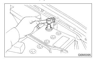
3) Disconnect front oxygen (A/F) sensor connector.
