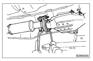
3) Separate rear exhaust pipe from muffler.
