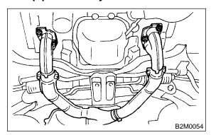
9) Remove bolt which installs front and center exhaust pipe assembly to hanger bracket.
