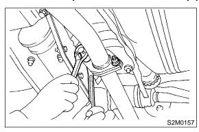
4) Remove rear exhaust pipe bracket from rubber cushion.
