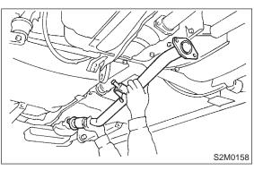
2) Install rear exhaust pipe to muffler.
