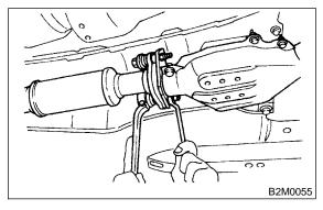
3) Separate rear exhaust pipe from muffler.
