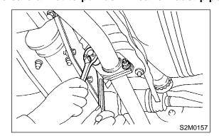
4) Remove rear exhaust pipe bracket from rubber cushion.
