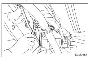
3) Install rear exhaust pipe to center exhaust pipe.
