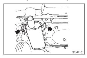
4) Remove front rubber cushion, and detach muffler assembly.
