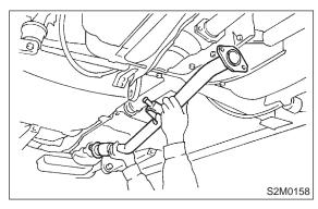
2) Install rear exhaust pipe to muffler.
