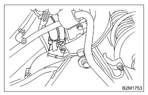
12) Disconnect evaporation hose from joint pipe.
