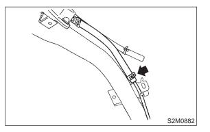
5) Install evaporation pipe to fuel filler pipe.
