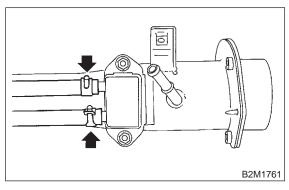
3) Connect evaporation hose to fuel filler pipe.
