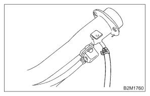
4) Disconnect evaporation hoses from shut valve.
