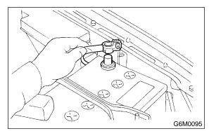
4) Disconnect connector from fuel pump.
