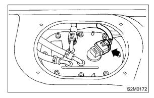
5) Move clips, and then disconnect fuel delivery hose (A), return hose (B) and jet pump hose (C).
