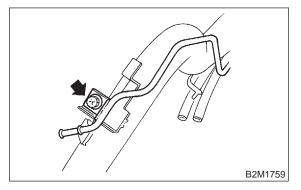
3) Disconnect evaporation hose from fuel filler pipe.
