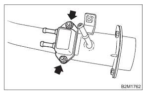
2) Connect evaporation hoses to shut valve.
