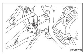
9) Connect evaporation hose to joint pipe.
