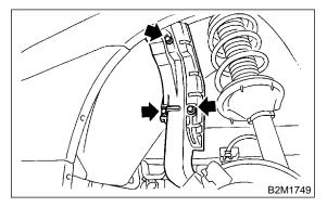
8) While releasing the under side of protector cover from hook, remove it.
