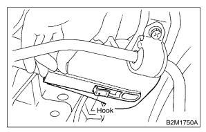
9) Disconnect evaporation hoses from pipes.
