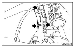
13) Tighten screws which install fuel filler pipe on filler lid open.
