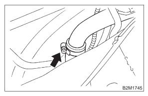
14) Remove fuel filler pipe to under side of vehicle.
