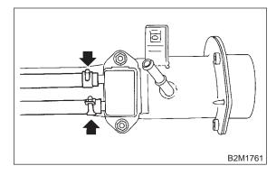
5) Remove shut valve from fuel filler pipe.
