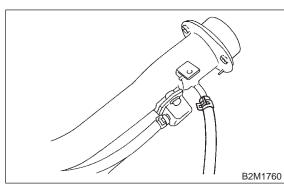
4) Connect evaporation hose to evaporation pipe.
