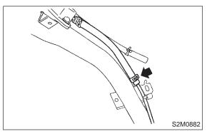
2) Remove bolt which installs joint pipe on fuel filler pipe.
