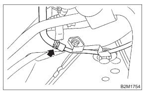
13) Loosen clamp, and disconnect fuel filler hose from fuel filler pipe.
