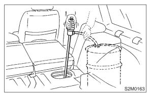
3) Remove screws which install fuel filler pipe on filler lid open.
