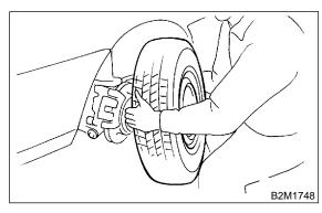
7) Remove bolts which install protector cover on body.
