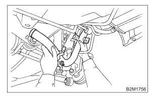
2) Connect fuel filler pipe into fuel filler hose.
