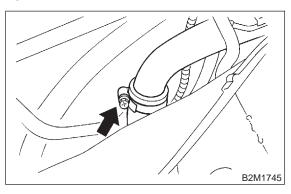
8) Install the two evaporation hoses to clip.
