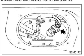
5) Move clips, and then disconnect fuel delivery hose (A), return hose (B) and jet pump hose (C).
