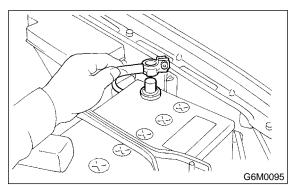
4) Disconnect connector from fuel pump.
