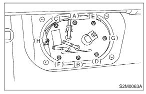
(4) Connect connector to fuel pump relay.
