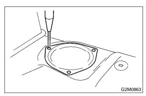
4) Disconnect connector from fuel sub level sensor, and disconnect jet pump hose.
