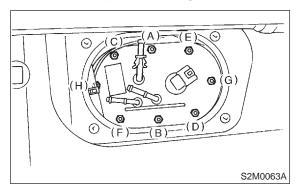
(5) Connect connector to fuel pump relay.
