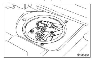
5) Remove bolts which install fuel sub level sensor on fuel tank.
