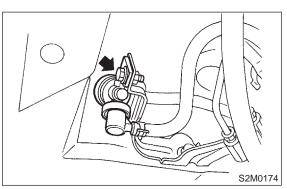
3) Disconnect hoses from roll over valve, and remove it from bracket.
