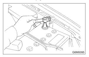
3) Disconnect fuel delivery hoses from fuel filter.
