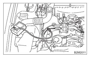
6) Check idle speed when unloaded. (With headlights, heater fan, rear defroster, radiator fan, air conditioning, etc. OFF)
