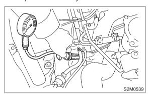
11) Perform at least two measurements per cylinder, and make sure that the values are correct.
