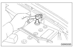
7) Start the engine, and measure oil pressure.
