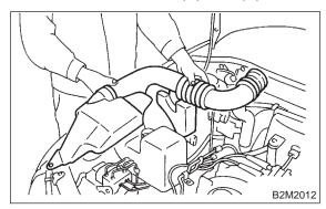
5) Loosen clamp which connects air cleaner case to throttle body.
