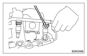
8) Tighten the two bolts which install fuel injector pipe on intake manifold.
