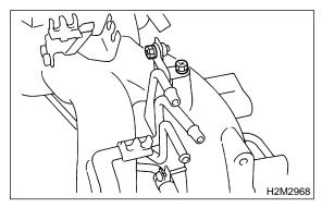
22) Remove bolt which installs injector pipe on intake manifold.
