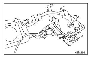
18) Install air assist injector solenoid valve to bracket.
