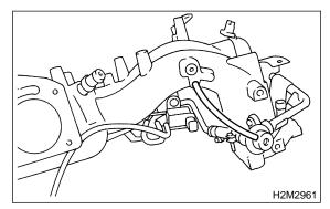
13) Disconnect connectors from fuel injectors.
