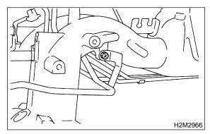
21) Remove the two bolts which hold fuel pipes on the left side of intake manifold.
