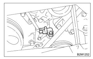
16) Disconnect connector from oil pressure switch.
