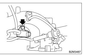
19) Remove bolt which installs injector pipe on intake manifold as shown in figure.
