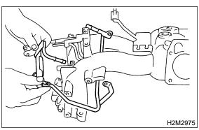
5) Connect left side fuel hose to injector pipe, and tighten clamp screw.
