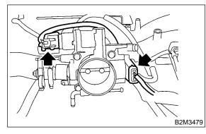
23) Connect air by-pass hose to throttle body.
