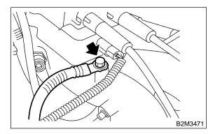
2) Disconnect connector from ignition coil and ignitor assembly.
