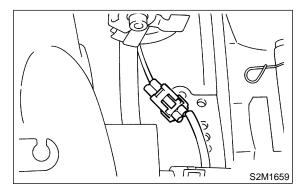
7) Connect connectors to engine coolant temperature sensor.
