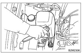
14) Connect accelerator cable (A).15) Connect cruise control cable (B). (With cruise control models)
