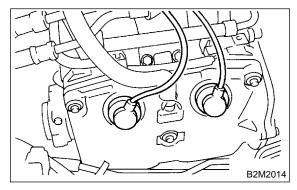
9) Disconnect PCV hose from intake manifold.
