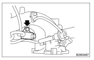
13) Connect hoses to purge control solenoid valve.
