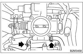
11) Connect PCV hose to intake manifold.
