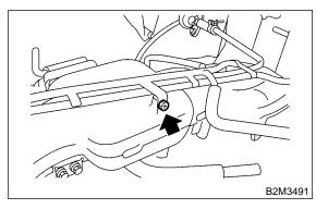
3) Connect right side fuel hose to injector pipe, and tighten clamp screw.
