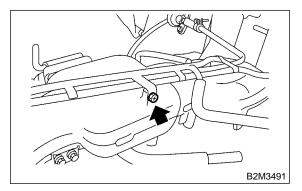
29) Remove fuel pipe assembly and pressure regulator, from intake manifold.
