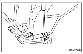
4) Install fuel injector pipe.
