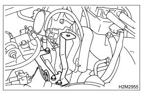
13) Disconnect connectors from engine coolant temperature sensor.
