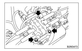
27) Connect connector to ignition coil and ignitor assembly.
