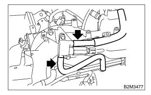
20) Connect connector to air assist solenoid valve.
