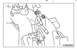
11) Tighten bolt which install injector pipe on intake manifold.
