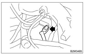
15) Disconnect air by-pass hose from purge control solenoid valve.
