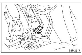
4) Connect connector to oil pressure switch.
