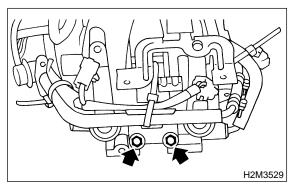
9) Tighten bolt which installs injector pipe on intake manifold.
