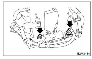
14) Disconnect connector from purge control solenoid valve.
