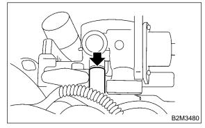
24) Install intake air temperature and pressure sensor.
