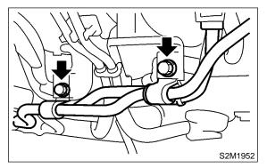
(3) Install power steering pump drive V-belt.
