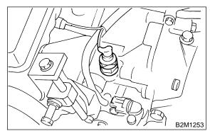
17) Disconnect connector from camshaft position sensor.
