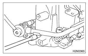
10) Tighten the two bolts which install fuel pipes on the left side of intake manifold.
