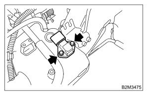
6) Disconnect connectors from throttle position sensor and idle air control solenoid valve.
