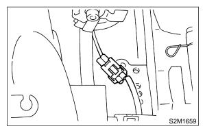
15) Disconnect connector from crankshaft position sensor.
