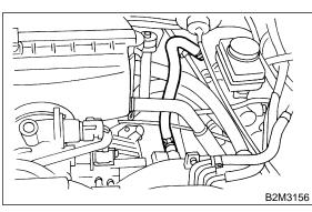
12) Remove air cleaner case stay RH and engine harness bracket, and disconnect engine harness connectors from bulkhead harness connectors.
