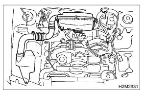
5) Disconnect accelerator cable (A).
