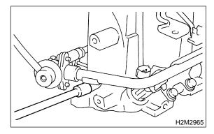
20) Remove bolt which installs injector pipe on intake manifold.
