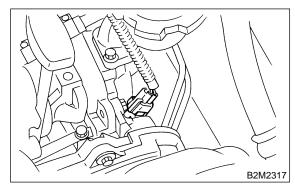
18) Disconnect fuel hoses from fuel pipes.
