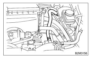
10) Connect engine coolant hose to throttle body.
