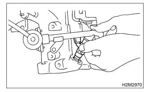
24) Disconnect air by-pass hoses from intake manifold.
