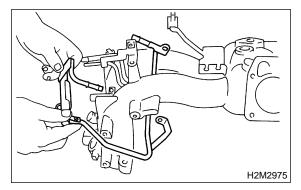
28) Remove bolt which installs fuel pipes on intake manifold.
