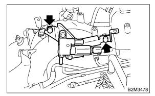
19) Connect air by-pass hoses to air assist solenoid valve.
