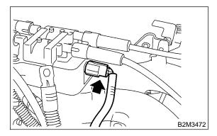
3) Remove ignition coil and ignitor assembly.
