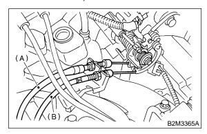
7) Remove power steering pump from bracket.(1) Remove resonator chamber.
