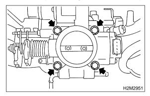
22) Connect connector to throttle position sensor and idle air control solenoid valve.
