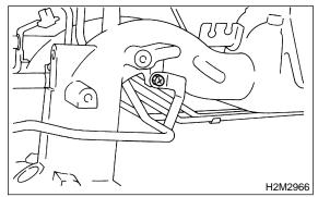
12) Install purge control solenoid valve.
