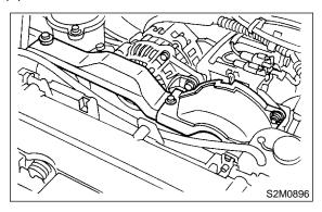
(6) Install resonator chamber.
