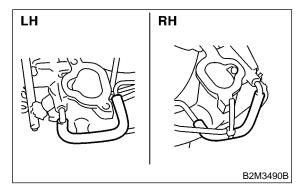
25) Loosen clamp which holds front left side fuel hose to injector pipe and remove the pipe from clamp.
