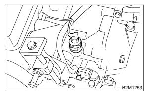
5) Connect connector to crankshaft position sensor.
