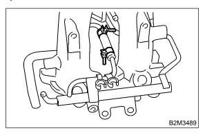
26) Loosen clamp which holds front right side fuel hose to injector pipe and remove the pipe from clamp.
