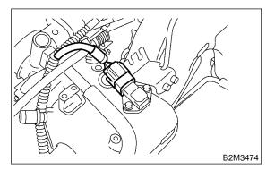
5) Remove intake air temperature and pressure sensor from intake manifold.
