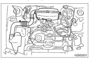
3) Disconnect connector from engine coolant temperature sensor.
