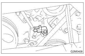
3) Remove crankshaft position sensor, and disconnect connector from it.
