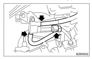
3) Remove air assist injector solenoid valve from intake manifold.
