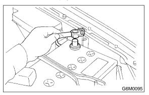
2) Disconnect connector from air assist injector solenoid valve and disconnect air by-pass hoses.
