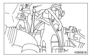
3) Take out purge control solenoid valve through the bottom of the intake manifold.
