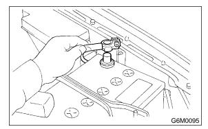
2) Remove bolt which holds bracket of main relay and fuel pump relay.
