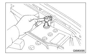
2) Disconnect connector from fuel pump relay.
