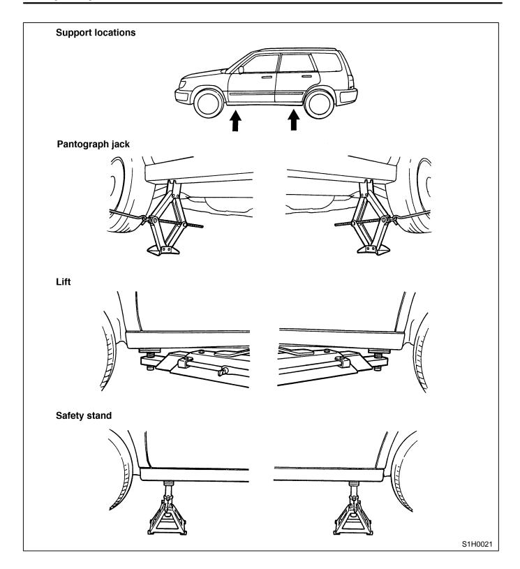
7. Lifting, Towing and Tie-down Points
