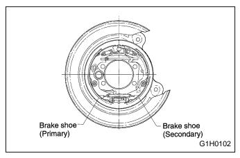
2) Check brake drum for wear, dents or other damage. If the inside surface of brake drum is streaked, correct the surface with emery cloth (#200 or more). If it is unevenly worn, tapered, or the outside surface of brake drum is damaged, correct or replace it.
