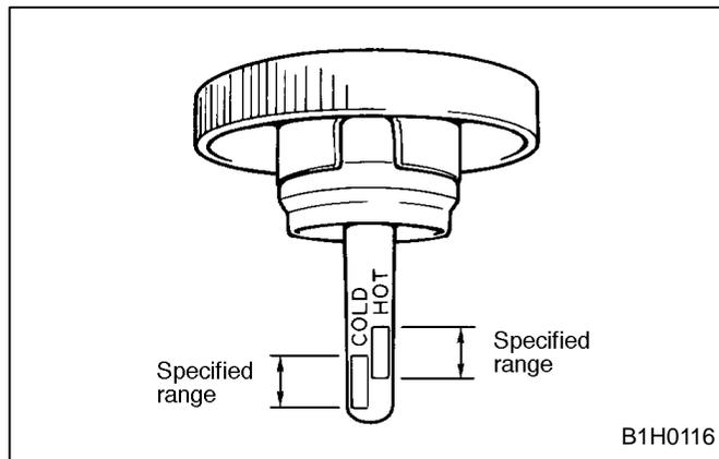
3) Fluid level should be maintained in the each specified range on the indicator of filler cap.
