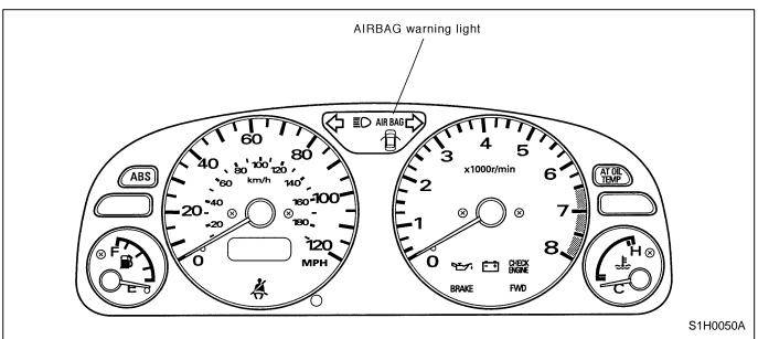
2) Turn the ignition switch ON, and connect the airbag diagnosis terminal of the service connector (located below lower cover) to the ground terminal.
