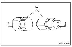
2) Visually inspect the O-ring surface, the O-ring mating surface, the threads and the connection points. If a defective part is found, replace it. The O-ring must sit square against the tube bead. If necessary, slide the O-ring into proper position with clean hands.
