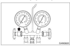
5) After 5 minutes, re-check the low-pressure gauge reading.
