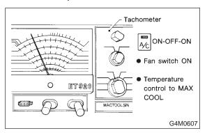
6) Raise engine rpm to approximately 1,500 rpm.
