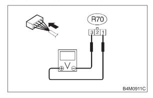
CHECK : Is the voltage between 4.75 and 5.25 V?
