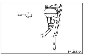
CHECK : Is the voltage between 3.7 and 4.1 V when G sensor is inclined forwards to 90°?
