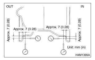
3) If rim runout exceeds specifications, remove tire from rim and check runout while attaching dial gauge to positions shown in figure.
