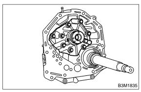
5) Remove the inner and outer rotor.
