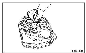
(3) If depth and/or side clearances are outside specifications, replace rotor assembly.
