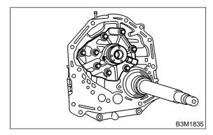
• Install the oil seal retainer and seal rings. After adjusting the drive pinion backlash and tooth contact.
