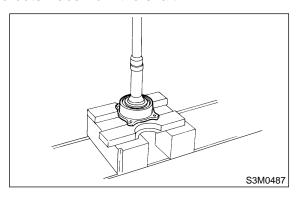
4) Using a press and ST, separate the front roller bearing from the shaft.
