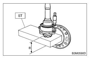
8) Determine the thickness "t" (mm) of the drive pinion shim.
