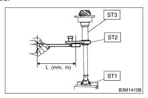
5) Measure the starting torque of the bearing. Make sure the starting torque is within the specified range. If out of the allowable range, replace the roller bearing.
