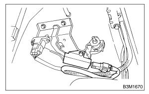
5) Install dropping resistor.
