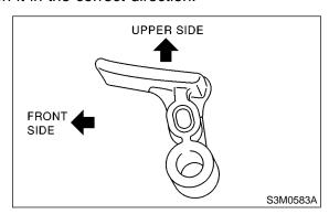
• Be careful to install the spring and button into the select lever grip in the correct direction.
