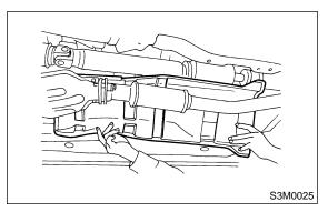
3) Disconnect cable from select lever and then remove cable bracket.
