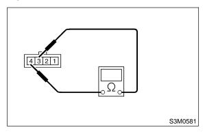
4) Connect lead harness to connector terminal of shift-lock solenoid, and apply battery power to check whether the solenoid operates.
